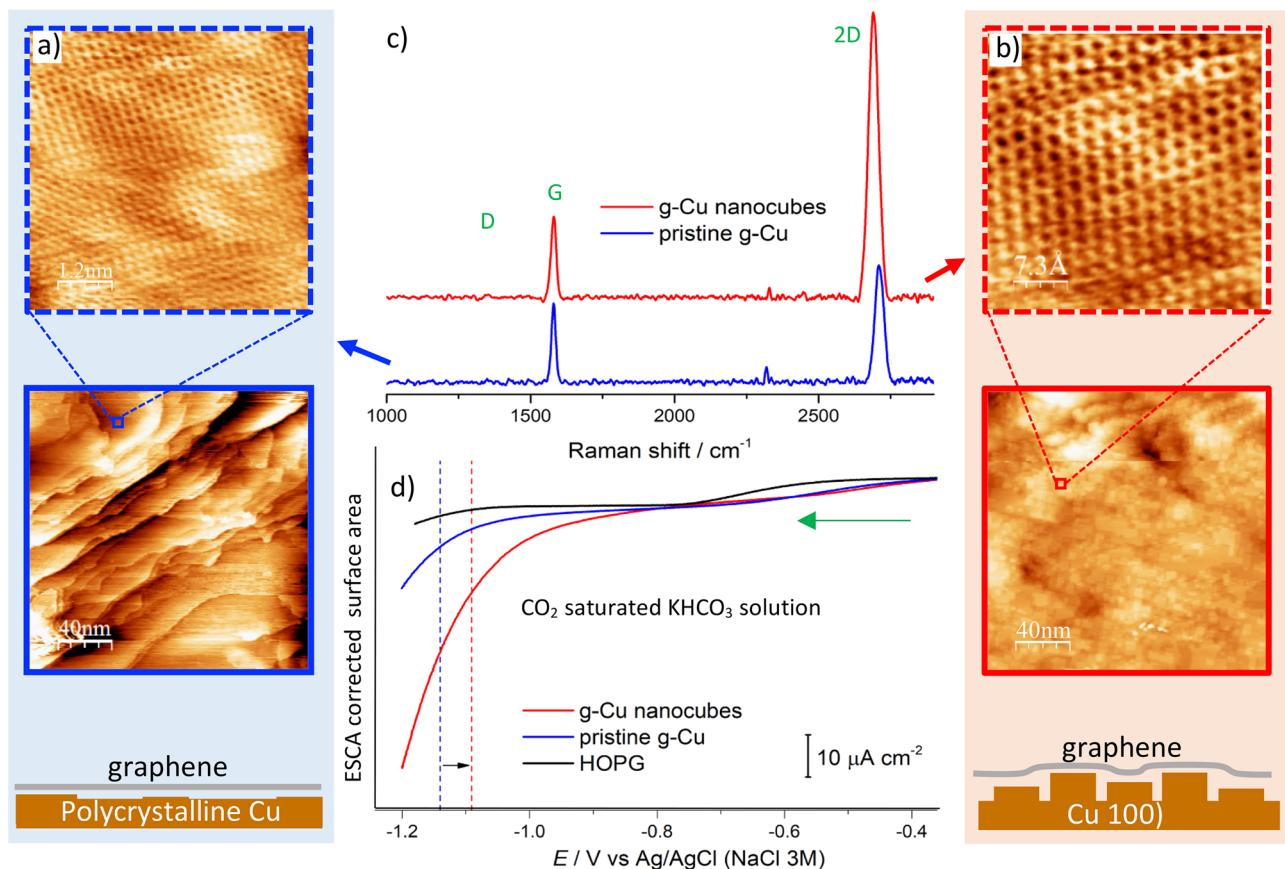
**Figure 3.** *Ex situ* STM images showing graphene (a) before and (b) after reconstruction to g-CuNCs.  $U_{bias} = 0.1$  mV,  $I = 10.5$  nA. (c) *Ex situ* Raman spectra of pristine g-Cu and g-CuNCs. The gray band highlights the wavenumber where the D band is usually observed. (d) ECSA-corrected linear sweep voltammograms obtained for pristine g-Cu, g-CuNCs, and HOPG.
